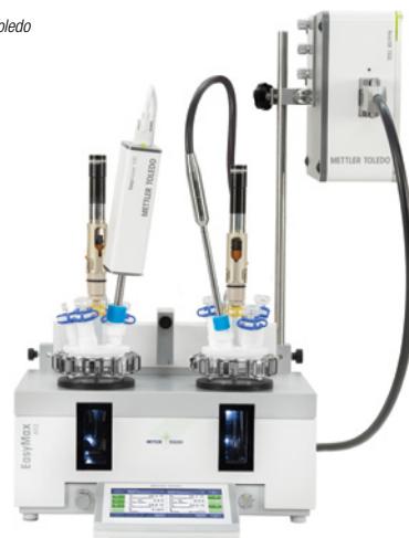
FIGURE 1. Shown here is a PAT-equipped Synthesis Workstation for Process Development and Optimization. For accelerated process knowledge, Easymax automated reactor is equipped with ReactIR in situ FTIR and ParticleTrack particle characterization PAT. Used in conjunction with Dynochem process modeling, the technology facilitates rapid development, optimization and scale-up of chemical reactions and crystallization processes
