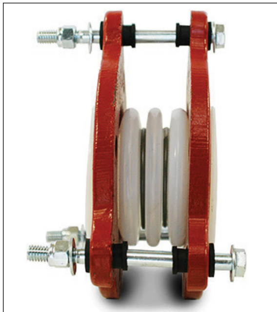
FIGURE 8. Control rods prevent the expansion joint from extending beyond its capabilities
