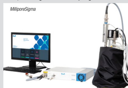
FIGURE 5. MilliporeSigma's ProCellis Raman Analyzer probe is immersed into the bioreactor, protected from external straylight with a light-proof fabric. The instrument is controlled by Bio4C PAT Raman software
